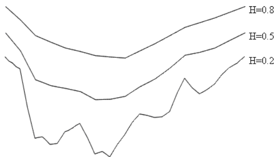
Figure 2: Generating a random fractal terrain. This picture shows a generated terrain profile as the randomness inverse-scale-factor H falls (as it gets smaller, randomness rises). The final “curve,” where H = 0.2 , looks strikingly like a stock price chart. Courtesy of http://www.gameprogrammer.com/fractal.html .
